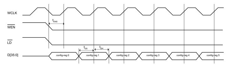
Figure 14. Configuration Register Read
